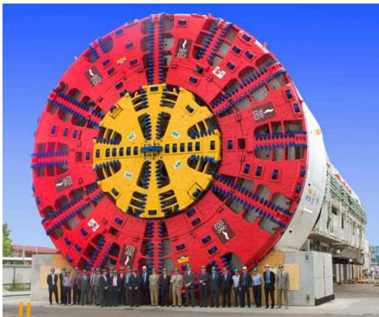
Figure 4-5. Herrenknecht EPB Shield S-300 mega tunnel boring machine [Herrenknecht, 2009].
