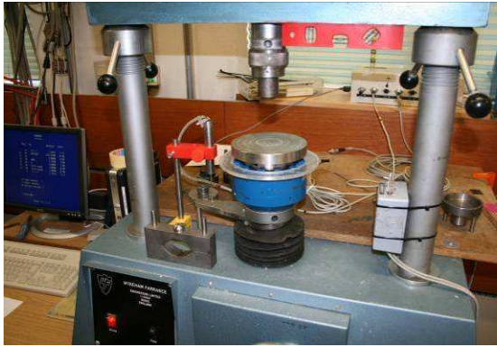
Figure 10-8. Test setup for Brazil test, includes a loading frame, a data logger, a load cell, a vertical strain gauge and a computer. Figure 10-9. Sample placed in between the two jaws and ready for testing.
