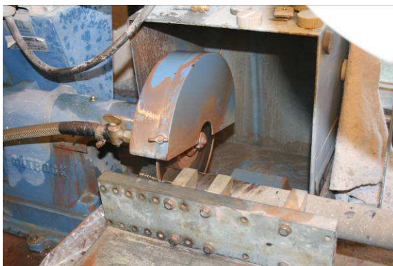
Figure 10-2. Core sample cut in diamond disc saw.
