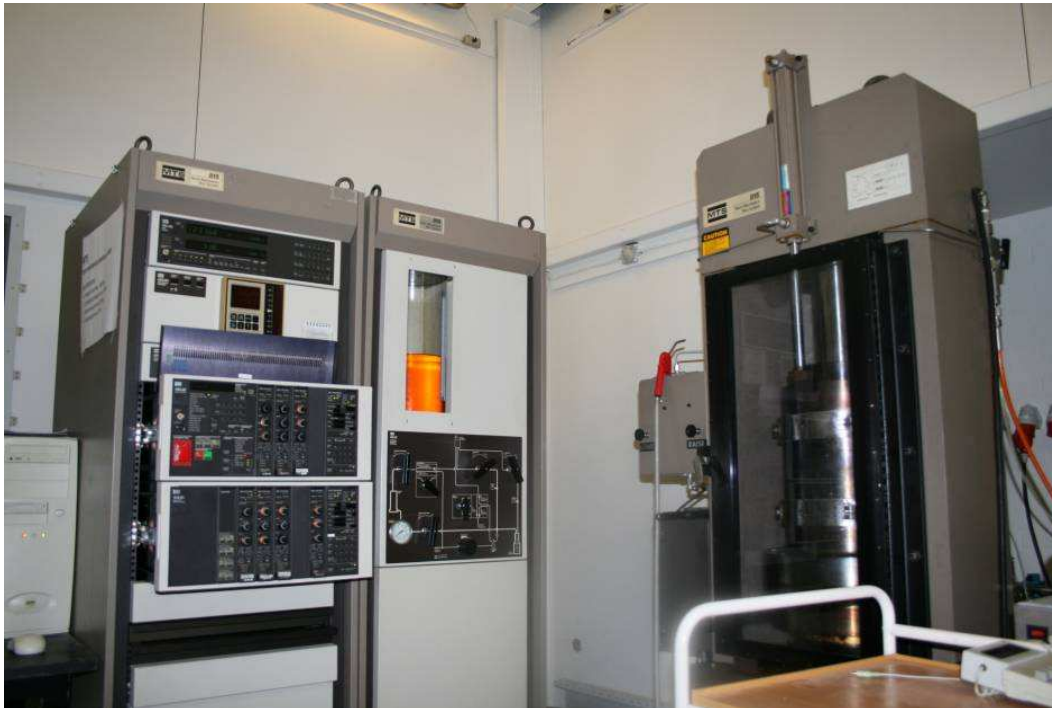
Figure 10-11. The MTS rock mechanics test system 815 at DTU used in the triaxial tests.
