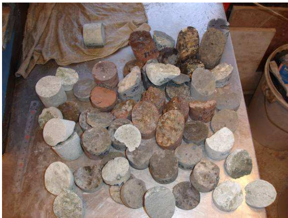
Figure 10-5. Cut of waste away during sawing of samples.
