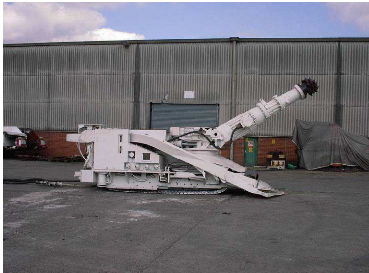
Figure 4-6. A Roadheader excavation machine [Dosco, 2009].
